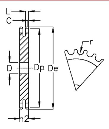
C = 6 D = 30 De = 589.5 Dp = 566.71 For chain size =  $2 \times 1 \frac{1}{4}$ For chain type =  $32 \times 1 = 87.4$
